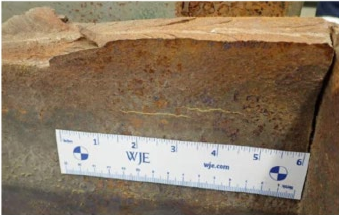
Figure 1. 2 1/4-inch thick plate side of fracture with cracks highlighted by yellow filings.
