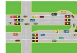
Thru-turns can help traffic turn left quicker and safer.
